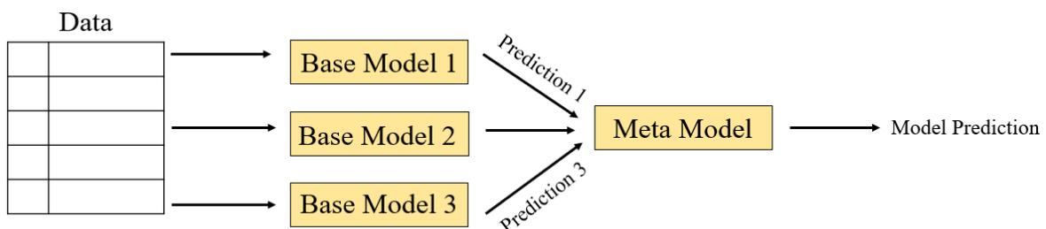
Figure 4. Stacking Algorithm
